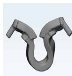
Figure 2) 3D printed jig after uniting the sub parts
